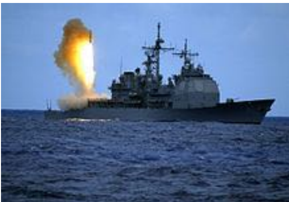
The Aegis Ballistic Missile Defense System. A RIM-161 Standard Missile 3 anti-ballistic missile is launched from USS Shiloh, a U.S. Navy Ticonderoga-class cruiser.
